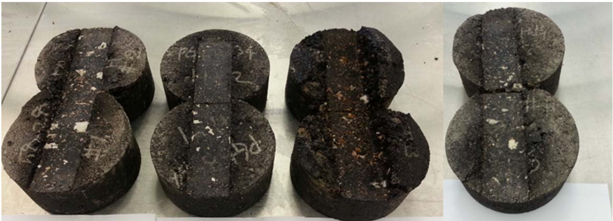
(a) Control Mix: PG58-28 (b) PG58-34 (c) PG58-28 w/ 0.6% Hydrogreen on total binder (d) PG58-28 w/ 0.75% Hydrogreen on total RAP/RAS
