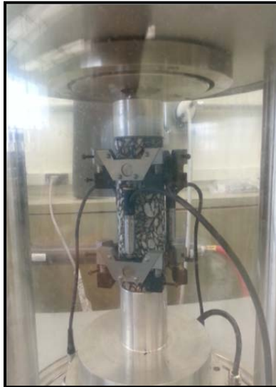
Figure 34. Small Scale PMFC Specimens for Dynamic Modulus Test.
