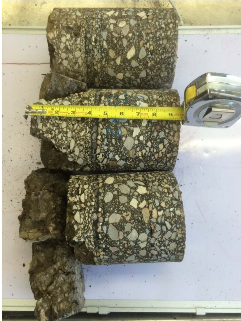
Figure 64. Cores Taken from Three Test Sections on US62.
