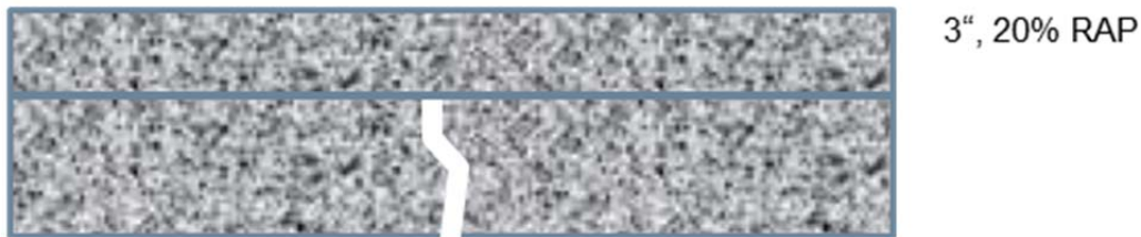
Figure 47. Schematic Diagram of the SH359 Pavement Structure.
